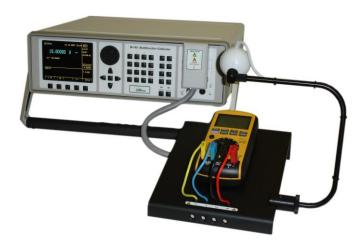
Automated Calibration of Multimeters using the digital camera and the software WinQbase.
