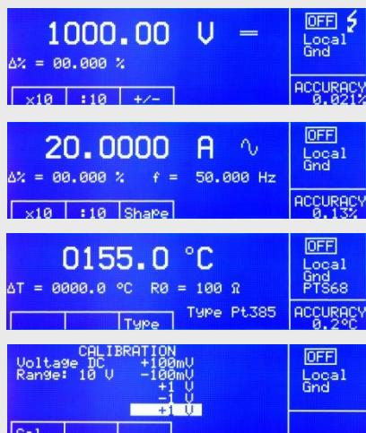
Presence of dangerous voltage over 100 V at the output terminals is indicated with „⚡” at the display and with beeping.
