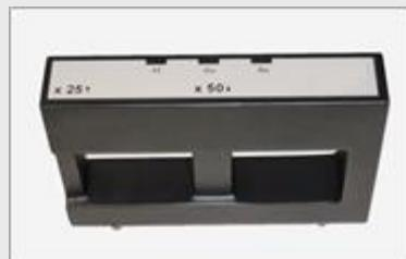
Option 140-50 Current coil with multiplying coefficient x25 and x50 is used for calibration of clamp amperemeters up to 1000 A at 50/60 Hz.
