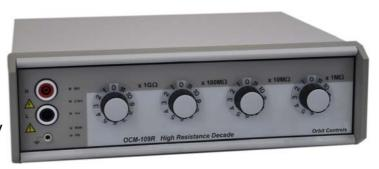
**OCM-109R** is a precise four digit high value resistance decade for testing and calibration of Megaohm-Meters and Testers for isolation resistances. It can also be used for testing and measuring of input impedances of signal conditioners and other applications in which resistance values of up to  $12~G\Omega$  are required. The maximum applied voltage is 5kV.
