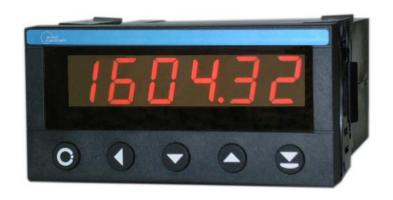
OC7171A-ABS is a six digit counter for connection to absolute coded signals from resolvers or linear displaycement lineals with Gray or binary coding. The instrument is designed for precision positioning or angular measurements. Single Turn or Multi Turn sensors with up to 64 serial Bits RS485, SSI or EnDat coding can be connected.
