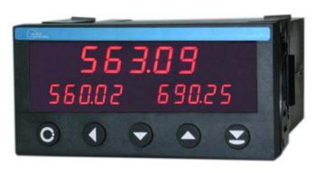
Model OC7171A-3D is a programmable counter with three displays. It can be programmed as a Quadrature bi-directional Counter, Up-Down Counter and Tachometer-Frequency Counter for industrial applications in connection with digital encoders, magnetic pick-ups and other industrial pulse sources. Integrated excitation is available for supplying of external sensors.
