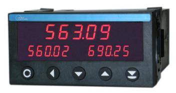
Model OC7171A-3D-3S is a programmable counter with three free scaleable displays. It can be programmed as a Quadrature bi-directional Counter, Up-Down Counter and Tachometer-Frequency Counter for industrial applications in connection with digital encoders, magnetic pickups and other industrial pulse sources. Integrated excitation is available for supplying of external sensors.
