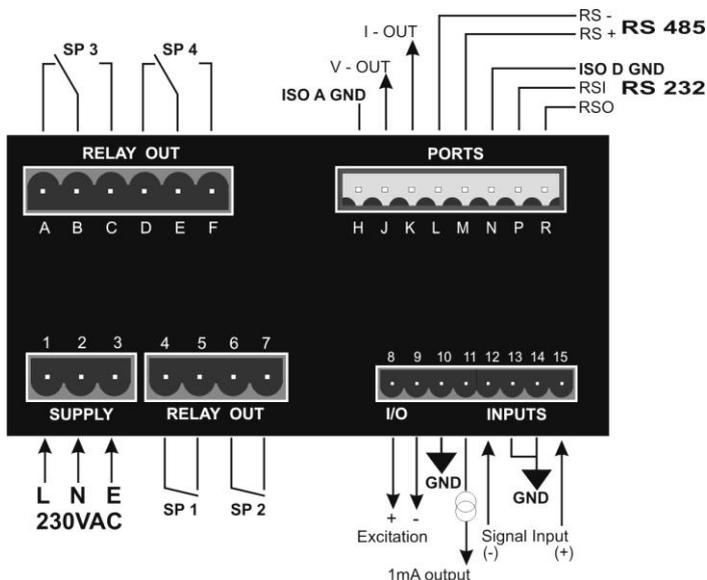
Standard instruments contain two Set Point Relays SP1, SP2, Supply 230VAC (115VAC) and adjustable excitation 5-24V.
