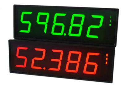
**OC557** is a 5 Digit programmable controller with 57mm green, red or yellow seven segments display units. The instrument is mainly designed for connection to process signals such as 0/4-20mA, and optionally 60mV to 300VDC or true RMS, RTD Sensors, Thermistors, Resistors, Potentiometers, Thermocouples and other industrial signal sources.
