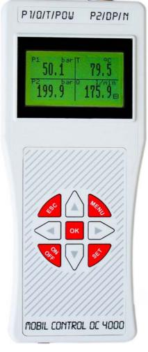
For measurements of fast Transients of the pressure sensor, eight memory slots are reserved for 8 individual transient measurements. The results are displayed as graphics at the front display.
