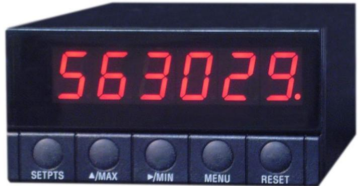
**INF8-C** is keypad programmable counter for use as a quadrature counter, up-down counter, or angular counter. The instrument is designed for fast positioning applications in connection with digital encoders, magnetic pick-ups and absolute code resolvers.
