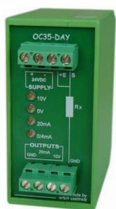
Ranges from 100 Ohm to 1 M-Ohm are available. The transmitter is calibrated on customer requirements, e.g. 0-25kOhm correspond to the output of 4-20mA.
