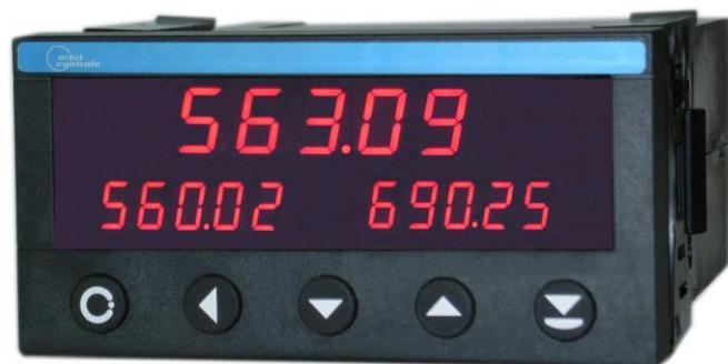
**Orbit Controls OC7171A-3D-SP** is a 5-digit counter with programmable functions for Quadrature Positioning Counter with bi-directional incrementing, Up-Down Counter and Tachometer-Frequency Counter. The instrument is designed for industrial applications in connection with digital encoders, magnetic pick-ups and other industrial pulse sources.
